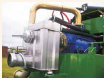
Warmth Exchanger on Pump Inlet
